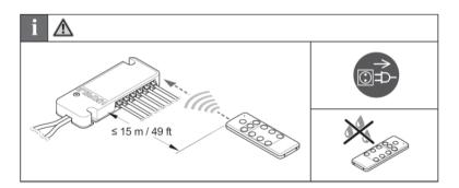
Multiple Wireless Remotes (hand held remotes [833.89.121] and remote switches [833.89.122]) can be paired to each Receiver Module.
