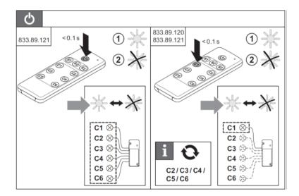
• Test the pairing by pressing the power button or individual zones (C1, C2 C3...) on and off. Note: C1 will turn all C1 lights on /off etc.
